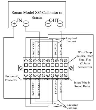
Figure 7.5: Analog Calibration Connections - Reverse Voltage Channel - (option)
