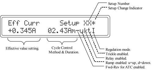
Figure 6.28: Main Screen Indicating the Setup Parameters
