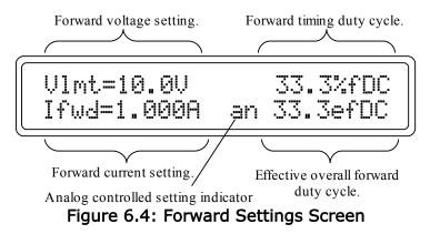
**Figure 6.4:** shows the settings for the forward voltage and current. The voltage and current settings are peak levels (On Time level). A small **`an**' is shown beside one or both settings indicates that the setting is being controlled by the optional analog input(s). Depending on
