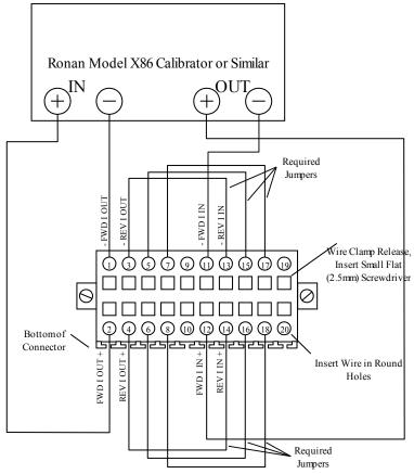
Figure 7.2: Analog Calibration Connections - Forward Current Channel
