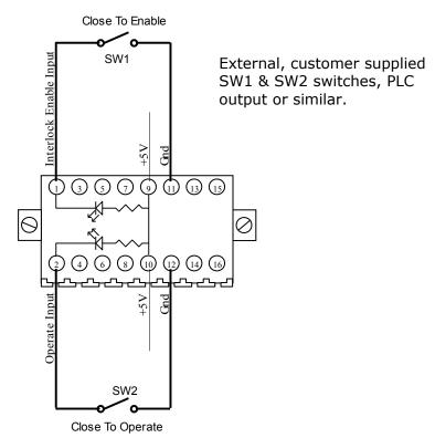
Figure 5.7: Digital Input Connections
