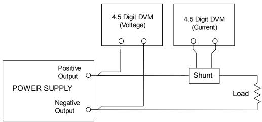
Figure 7.1: Output Calibration Connections
