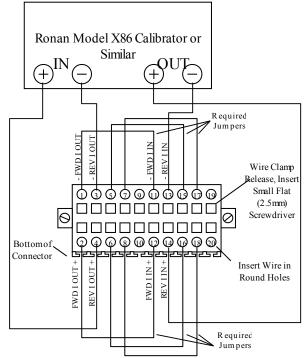
Figure 7.3: Analog Calibration Connections - Reverse Current Channel - (option)
