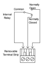
Figure 5.9: Relay Output Connector
